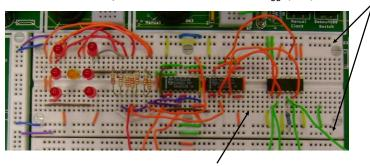
Vertical five hole strips used to connect up components
